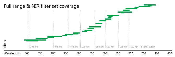
Sense wavelength coverage with full range and NIR filter sets installed.
